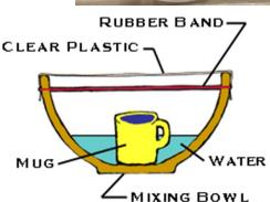
Add water to the large bowl until it is about a quarter full, place the empty mug in the center of the bowl without splashing any water into it. Cover the top of the bowl tightly with plastic wrap and tie the string or place the rubber band around the bowl to keep the plastic wrap in place. Place the bowl in a sunny location and watch the bowl to see what happens! To speed up the process use warm water and/or move the bowl to a shady spot after it has been in the sun for some time.
