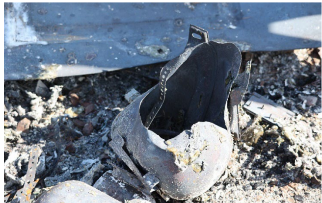
Figure 2.b.8. This propane tank, utilized to fuel a grill, was exposed to high amounts of radiant heat and eventually direct flame contact, as the home it was adjacent to burned, causing the gas to ignite and spread the fire further. (Source: Eli Loftis, Okanogan CD, 2023)
