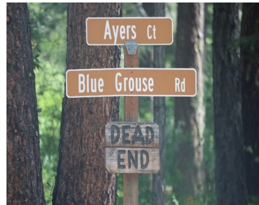
Figure 1.b.11. Address and road signage across the county is not cohesive and varies vastly in quality and utility. In this example the road signage is sufficient, but the non-reflective "DEAD END" sign would not be easily visible to fire responders and firefighters during an emergency wildfire event. (Source: Eli Loftis, Okanogan CD, 2024)
